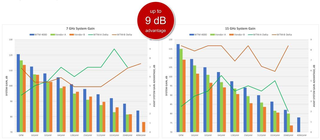
WTM 4000 System Gain outperforms most other radios in its Class
